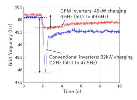
Figure 4: Verification of actual equipment when recharging batteries. Credit: Toshiba Corporation News Releases
