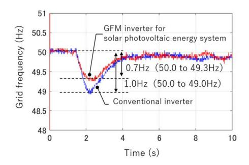
Figure 3: Verification of photovoltaic power generation applying the GFM inverter and a diesel synchronous generator with an internal combustion engine.
