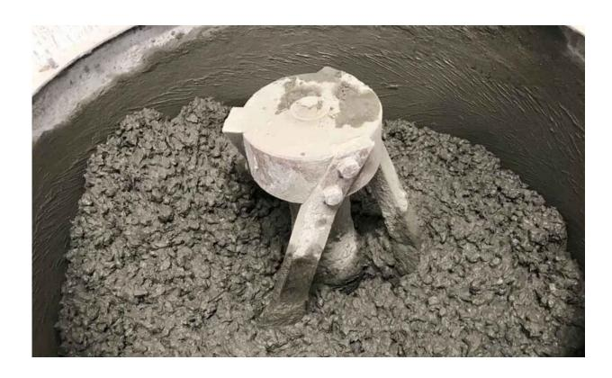
Concrete mixing using recycled tyre rubber particles for the complete replacement of traditional coarse aggregates. Credit: Mohammad Islam, RMIT
