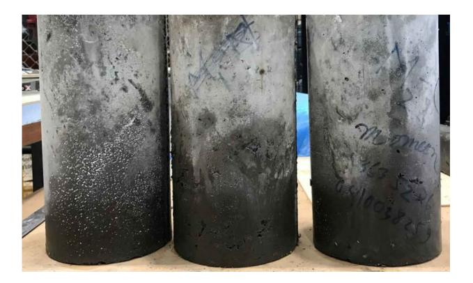
The RMIT team's new casting technique generates structural lightweight concrete from used tyre rubber. Credit: Mohammad Islam, RMIT
