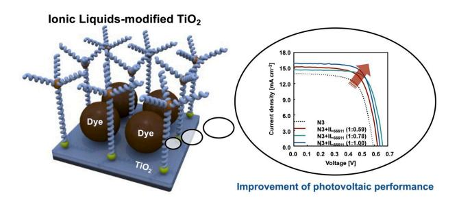
By modifying the surface of the oxide electrode with molten ionic salts, one can prevent the clumping of dye molecules without significantly impacting their coverage. This simple modification greatly improves the energy-conversion performance of dye-sensitized solar cells, find researchers from NITech, Japan in a new study. Credit: Tomohiko Inomata from NITech, Japan
