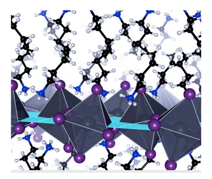
Hybrid perovskites are like molecular baklava with alternating metal-based inorganic layers and carbon-based organic layers. Interactions in the organic layer can tune distortions in the inorganic component and boost the efficiency of
