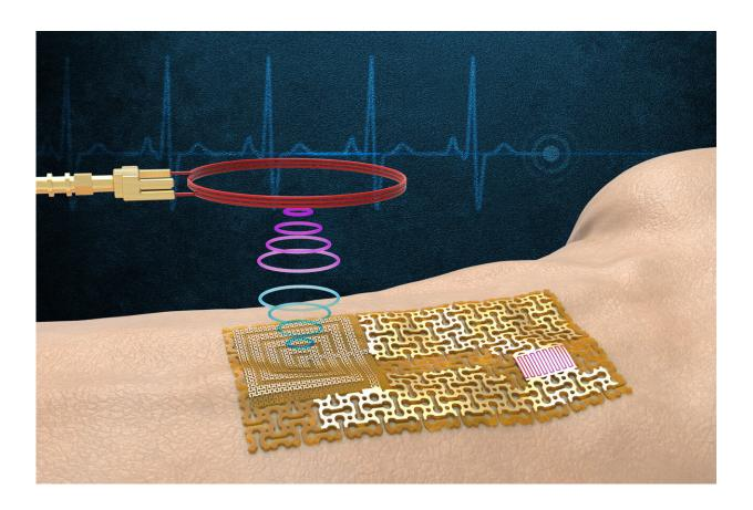
MIT engineers fabricated a chip-free, wireless electronic "skin." The device senses and wirelessly transmits signals related to pulse, sweat, and ultraviolet exposure, without bulky chips or batteries. Credit: Massachusetts Institute of Technology
