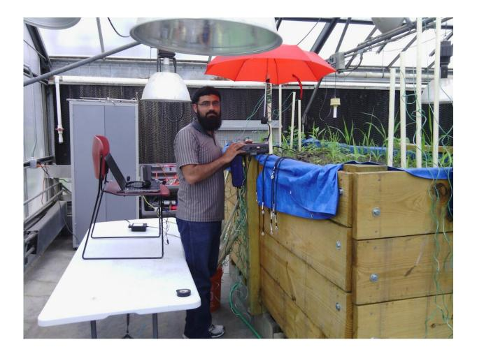
Abdul Salam takes measurements in a test bed at Purdue University to determine the optimum operating frequency for underground antennas. Credit: Abdul Salam, CC BY-ND
