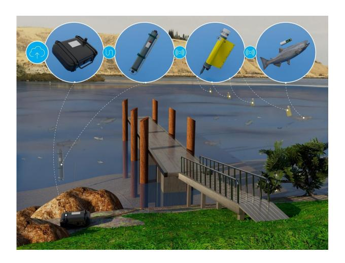
Researchers at Pacific Northwest National Laboratory have developed a receiver that can transmit near-real-time information on fish tracking to inform decisions about dam operations that support fish passage. Credit: Cortland Johnson | Pacific Northwest National Laboratory
