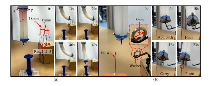
Object manipulations performed by our soft robot. RDSR completed pick-and-place tasks with large workspace precise operation. (a) The objects were placed near the boundary of the workspace (task1). (b) An object with a small diameter of 8mm was placed (task2). Credit: Wang et al.
