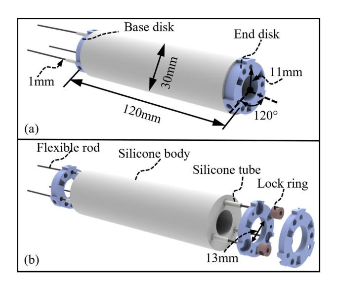
Structure of the rod-driven soft arm. (a) Design overview. (b) Exploded view. Credit: Wang et al.
