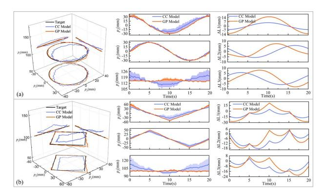
Trajectory tracking performances of the open-loop control based on CC and GP model. (a) Case for circular path. (b) Case for square path. Credit: Wang et al.
