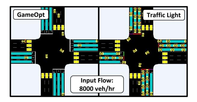
Image showing how GAMEOPT works compared to traffic lights. The light blue regions denote the control zone. The team showed that at identical input traffic flow levels, their approach outperforms even traffic light infrastructure, resulting in less queues and enabling smooth traffic flow. Credit: Suriyarachchi et al.
