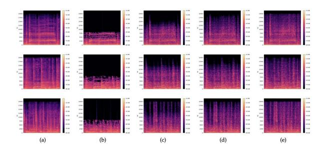
Spectrograms of (a) original audio excerpts, (b) corresponding 32kbit/s MP3 versions, and (c), (d), (e) restorations with different noise z randomly sampled from N (0,I). Credit: Lattner & Nistal.
