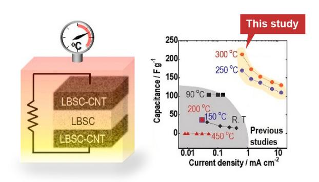
Bulk-type symmetric all-solid-state capacitor, with a LBSC SE layer between two electrode layers of an LBSC-CNT composite (left), showed low resistance and were operable at 100–300 °C (right). Credit: Hayashi, Osaka Metropolitan University
