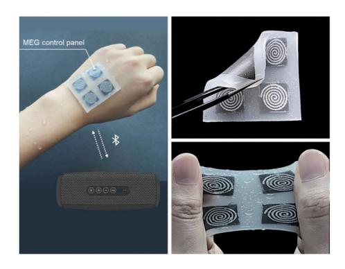
(Left) Photo of the magnetoelastic sensor array, which conforms to human skin and can function even when exposed to liquid. It can interact with a music speaker's command components: play, pause, next, and previous. (Right two) The self-powered magnetoelastic sensor array is rollable and stretchable. Credit: The Jun Chen Research Group at UCLA: junchenlab.com
