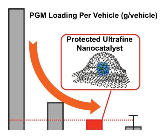
The authors' graphene-wrapped alloy yielded extraordinary results:75 times more catalytic activity65% more powerabout 20% more catalytic activity at the expected end of the fuel cell's lifeabout 35% less loss of power after testing that simulates 6,000 to 7,000 hours of use, beating the target of 5,000 hours for the first time. Credit: Huang Group UCLA
