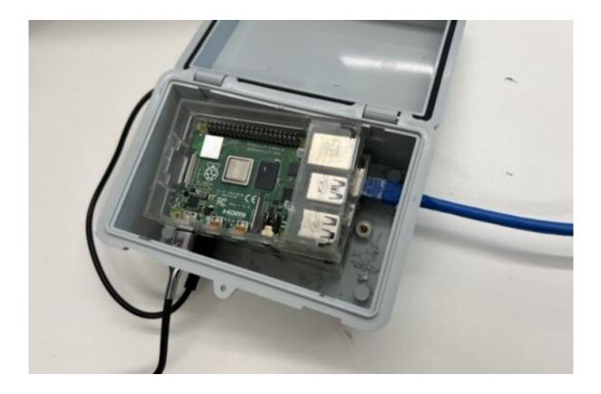
For the Sydney Harbour Tunnel test UNSW researchers placed a series of lowcost Wi-Fi transmitters and receivers, running on Raspberry Pi and installed in a waterproof enclosure, along the roadway to detect the change in signals caused by fire and smoke. Credit: Aruna Seneviratne
