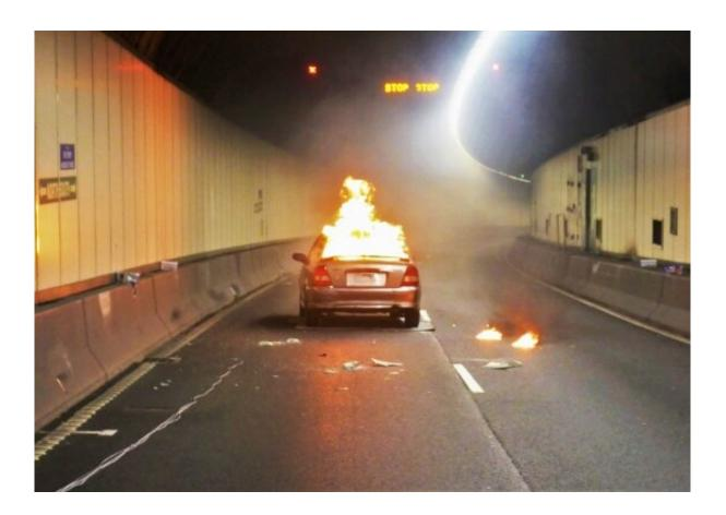
Wi-Fi transmitters and receivers were set up to monitor readings from this controlled test explosion of a car in the Sydney Harbour Tunnel. Credit: Aruna Seneviratne
