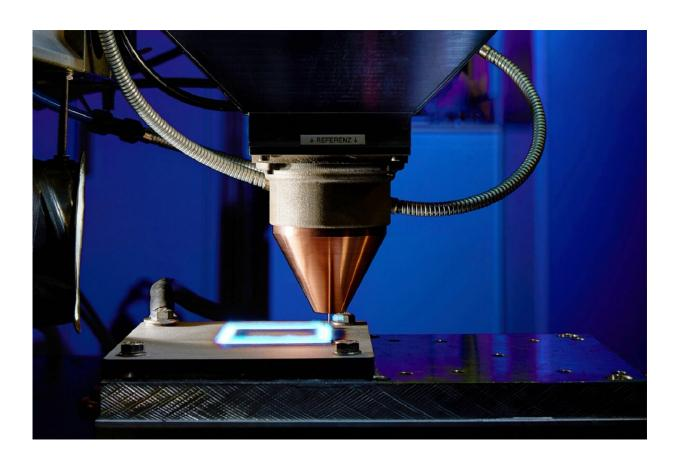
The new COLLAR Hybrid Additive Manufacturing process relies on a combination of arc and laser deposition. Credit: Volker Lannert
