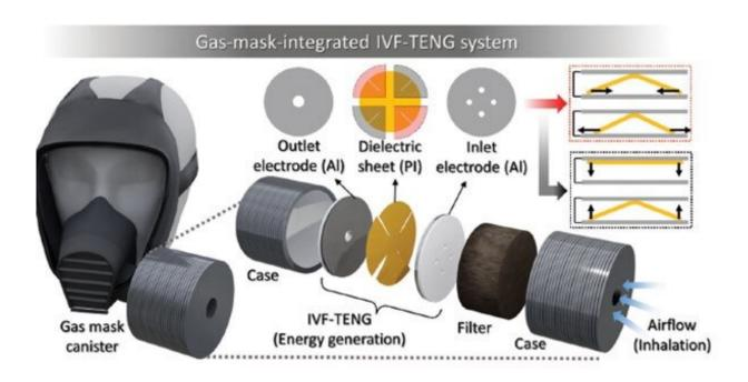
In a new study, Chung-Ang University researchers design a high-power and high output triboelectric nanogenerator (TENG)-based sensor that can be powered by breathing. The researchers integrated this device into a gas mask to create a self-powered hybrid sensor that detects breathing patterns and harmful chemicals. Credit: Prof. Sangmin Lee from Chung-Ang University, Korea
