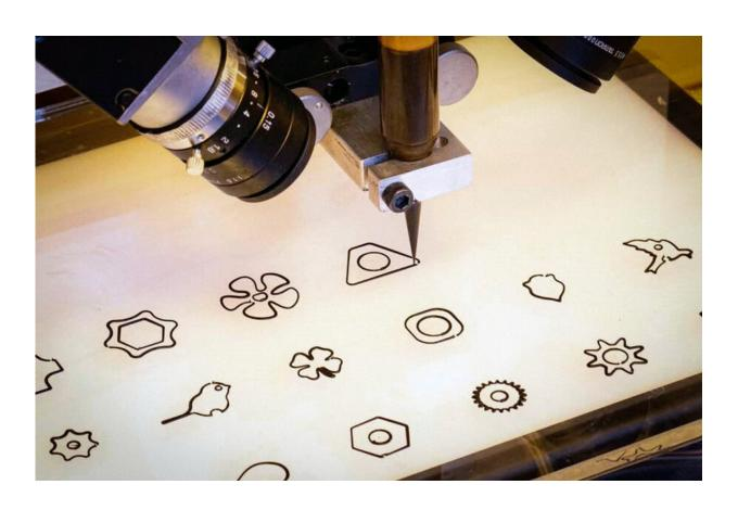
MIT researchers have trained a machine-learning model to monitor and adjust the 3D printing process in real-time. Credit: Massachusetts Institute of Technology
