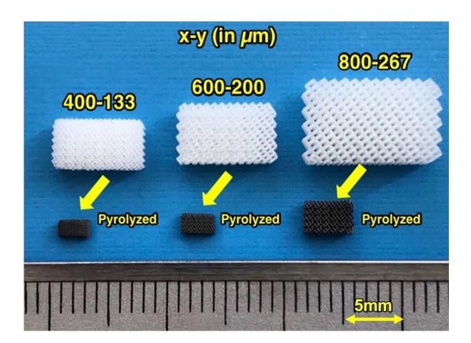
The 3D-printed lattices were prepared in three sizes. Carbonization through pyrolysis shrunk the electrode and increased its performance. Credit: Tohoku University
