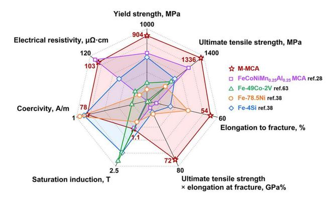
Comparison of the mechanical and functional property spectra of the new multicomponent alloy. Credit: *Nature* (2022). DOI: 10.1038/s41586-022-04935-3
