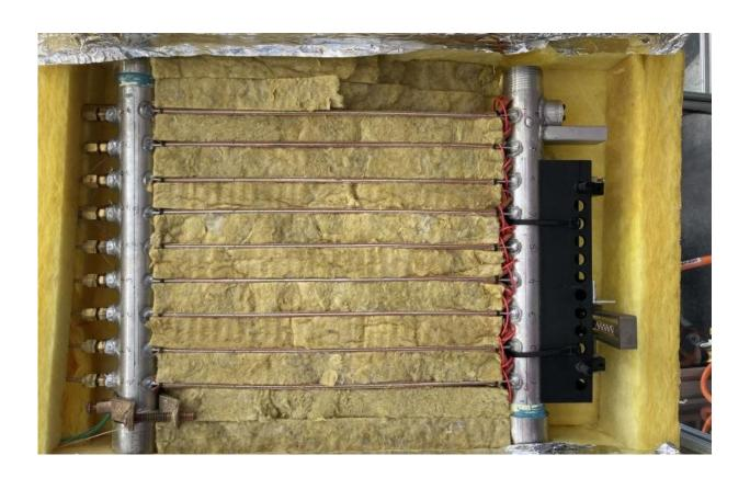
Oak Ridge National Laboratory researchers developed a device called a piezoelectric-driven magnetic actuator, or PEDMA, that can be inserted into the header of a microchannel heat exchanger to keep refrigerants flowing evenly and the HVAC unit running efficiently. Credit: ORNL, U.S. Dept. of Energy
