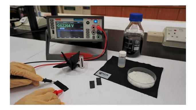
The new moisture-driven electricity generation device invented by NUS researchers capitalises on the difference in moisture content of the wet and dry regions of the carbon-coated fabric to create an electric current. Sea salt is used as a moisture absorbent for the wet region. Credit: National University of Singapore
