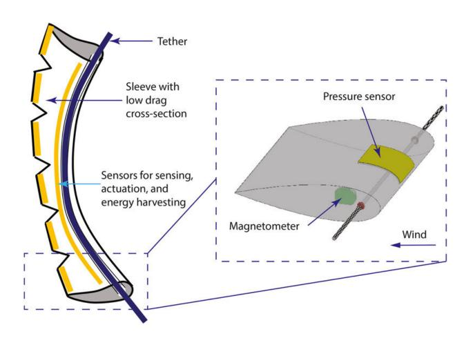
Notional schematic of a low-drag, smart tether system. The inset shows the concept of an airfoil-shaped anemometer instrumented with a conformable pressure sensor and a magnetometer for wind speed and direction measurements, respectively. Credit: Arun K. Ramanathan et al, *Frontiers in Materials* (2022). DOI: 10.3389/fmats.2022.904056
