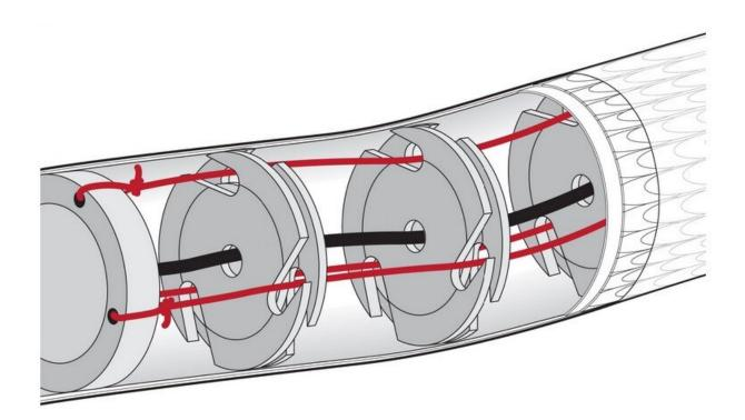
Threads running through the robot's "body" attach to a thicker disk at the end of each body segment. These threads are pulled to control individual segments of
