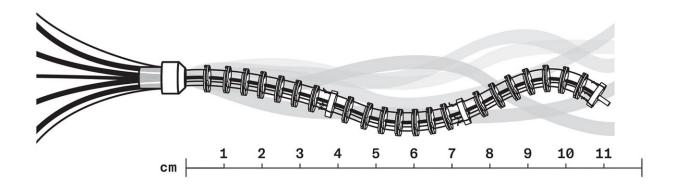
The "tendon-driven" continuum robots depicted here are, in real life, about seven millimetres in diameter and are built in sections that can range in length from 15 to 70 millimetres. Other models can be even narrower. All exhibit a tentacle-like motion. Credit: University of Toronto
