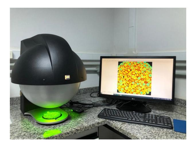
Multispectral images based on reflectance and autofluorescence are processed using mathematical models. Credit: Winston Pinheiro Claro Gomes
