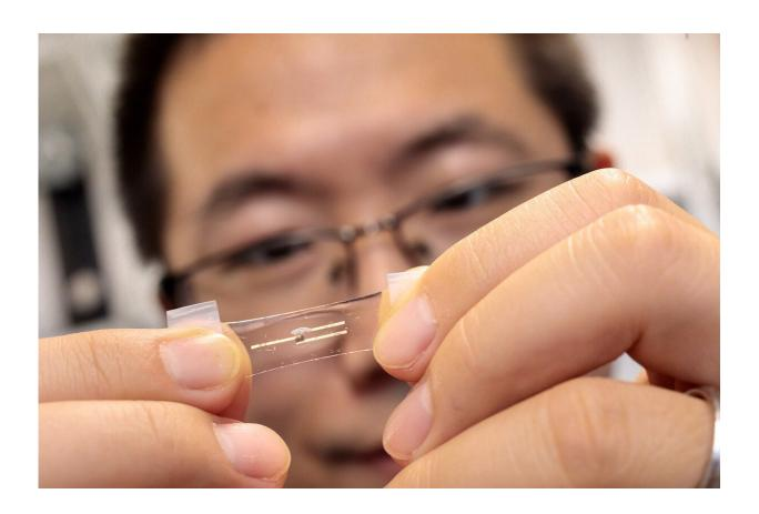
The wearable neuromorphic chip, made of stretchy semiconductors, can implement artificial intelligence (AI) to process massive amounts of health information in real time. Above, Asst. Prof. Sihong Wang shows a single neuromorphic device with three electrodes. Credit: John Zick
