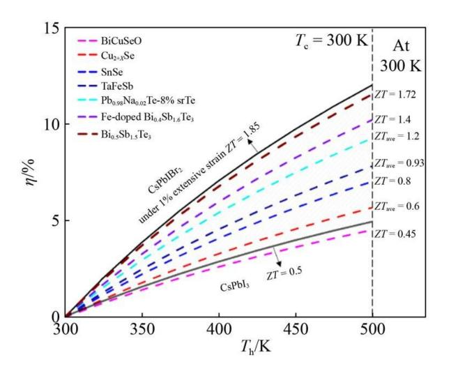
Thermoelectric energy conversion efficiency of inorganic halide perovskites compared with other thermoelectric materials. Credit: HIGHER EDUCATION PRESS LIMITED COMPANY
