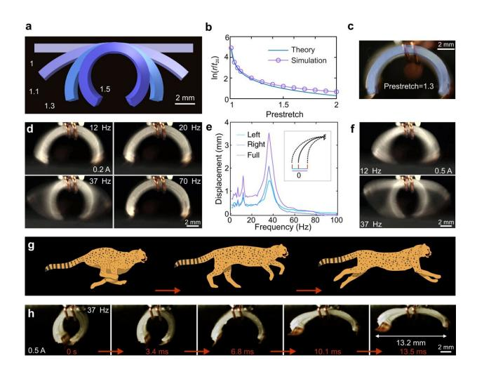
Design and characterization of small-scale SEMRs. a Simulated shape of the bilayer film with different prestretches: 1.0, 1.1, 1.3, and 1.5. b Simulated and calculated radius of the bilayer film as a function of the applied prestretch. c Superimposed pictures of the experimental and simulated SEMR shapes (side view) with a prestretch of 1.3. d Snapshots of the SEMR vibrations for 0.2 A
