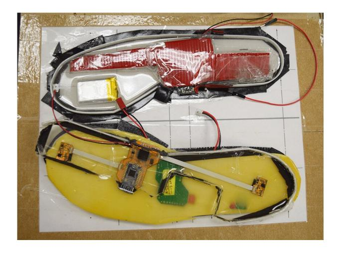
The smart insoles collect data from the toe-tapping test and transfer the information to a phone application. Credit: Texas A&M Engineering
