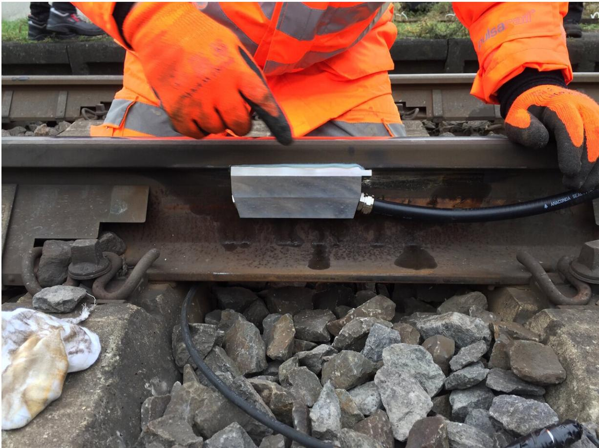
The SAFETRACK project's sensors can pick up vibrations on the railway track and identify where on the track the sound originates and what could have caused it. Credit: © NGRT SL
