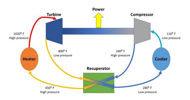
A diagram of Sandia National Laboratories' simple closed-loop Brayton cycle test loop. The working fluid being compressed, heated and expanded to produce power is supercritical carbon dioxide. Supercritical carbon dioxide is a nontoxic, stable material that is under so much pressure it acts like both a liquid and a gas. Credit: Sandia National Laboratories
