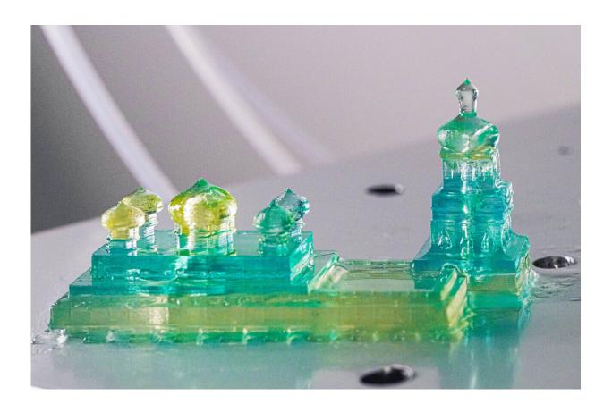
A model of Kyiv's Saint Sophia Cathedral in the blue and yellow of the Ukrainian flag, made using the iCLIP method for 3D printing, which allows for the use of multiple types – or colors – of resin in a single object. Credit: William Pan
