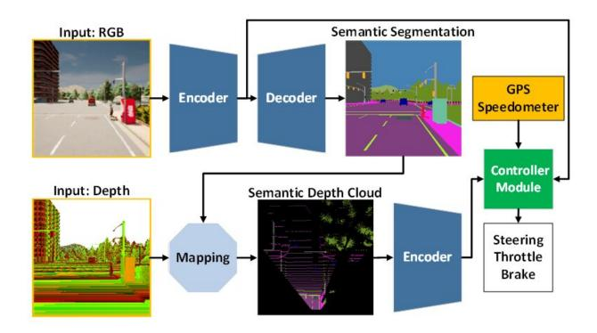
The AI model architecture is composed of the perception module (blue) and the controller module (green). The perception module is responsible for perceiving the environment based on the observation data provided by an RGBD camera. Meanwhile, the controller module is responsible for decoding the extracted information to estimate the degree of steering, throttle, and braking. Credit: Toyohashi University of Technology
