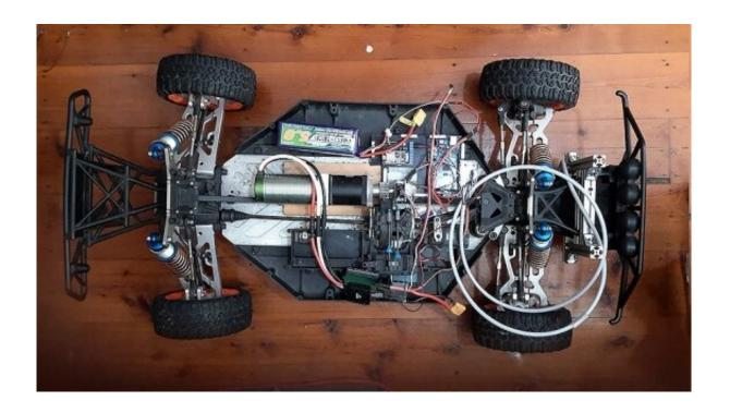
The car is equipped with multiple accelerometer and load cells to measure the dynamic response of the vehicle once it is moving over the bridge. Credit: UNSW
