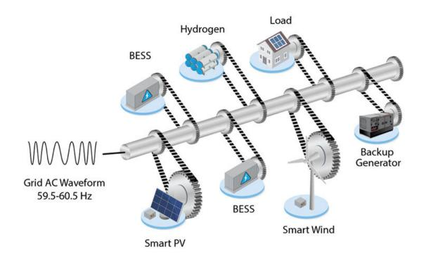
NREL's communication-less microgrid method allows grid frequency to vary across a wider range than normal. Devices watch the frequency and adjust their power output according to the frequency's changes. Credit: NREL
