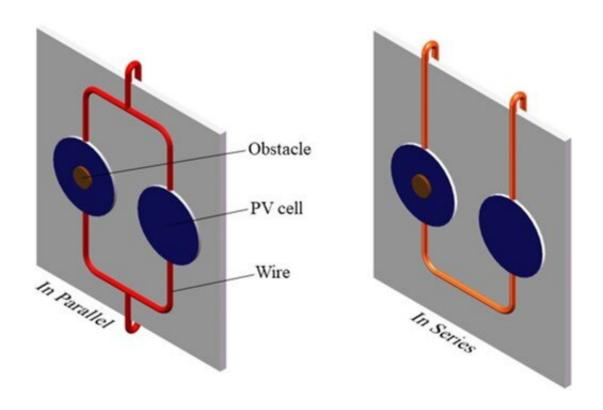
Two solar cells connected in parallel (left) and in series (right) with an obstacle creating shade (brown). Shady conditions caused more power loss in series systems. Credit: Guo et al.
