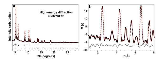
(a) Rietveld refinement of N70. Black circles are data points, the red line is the fit, and difference is shown beneath. Rw for the fit is 3.16. The upper ones are the allowed hkl for Ni and the lower for NiO. (b) Fit of the PDF of the N70 sample using Ni and NiO, with Ni contributing nearly all the fit intensity. Black circles are data points, the red line is the fit, and difference is shown beneath. Credit: *Applied Energy* (2022). DOI: 10.1016/j.apenergy.2022.119461
