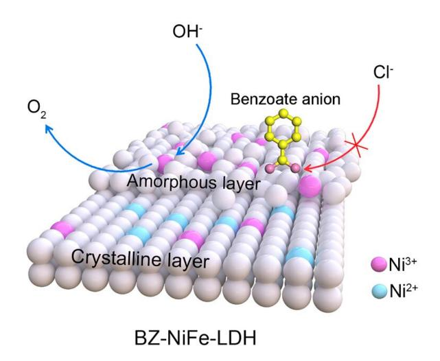
The picture illustrates the structure of the BZ-NiFe-LDH/CC material and how hydroxides penetrate the amorphous layer to react, while chlorides are repelled. Credit: *Nano Research Energy*
