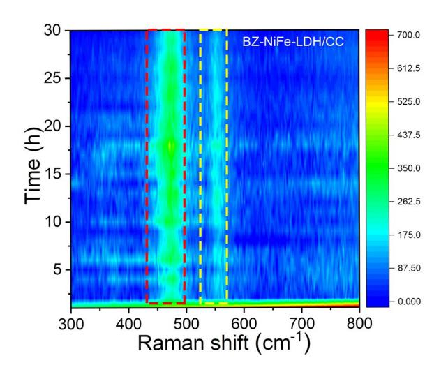
Spectroscopy imaging demonstrates the phase transition of OH- into oxygen through the newly developed electrode material of benzoate-nickel-iron-layered double hydrides on carbon cloth (BZ-NiFe-LDH/CC). Credit: *Nano Research Energy*
