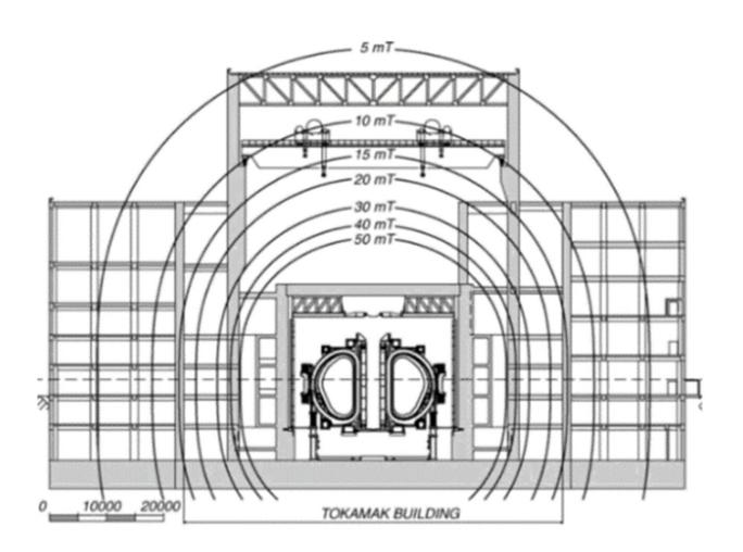
Magnetic field distribution around Tokamak. Credit: HUANG Ya
