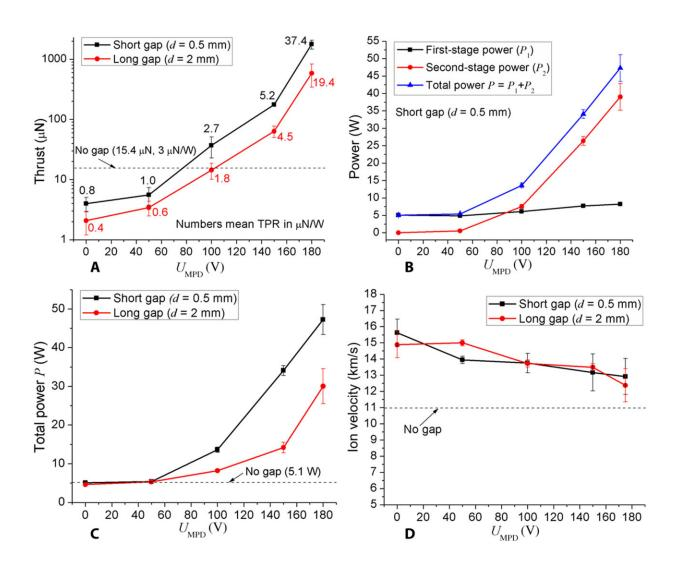
Experimental results of the  $\mu$ CAT-MPD thruster performance characterization. Thrust (**A**), power in both stages for the short gap (**B**), total power for the long and short gaps (**C**), and ion velocity (**D**) versus the second-stage (MPD) voltage  $U_{\text{MPD}}$ . Ti cathode, Cathode material is titanium. *Science*
