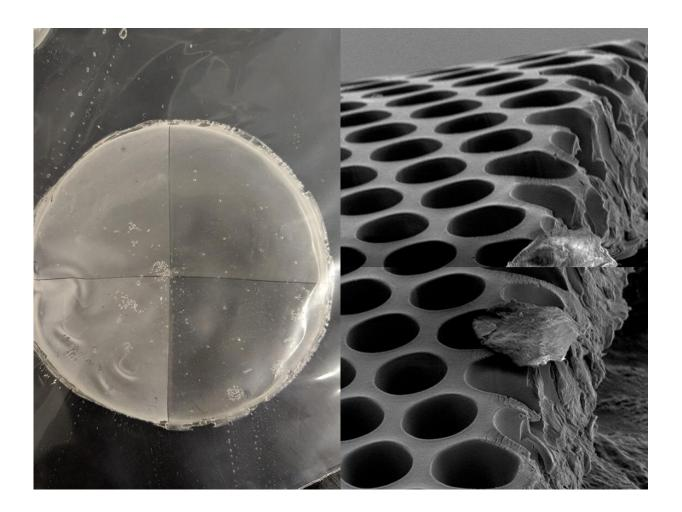
Penn State researchers will fabricate membranes with different surface pattern geometries and sizes to use in membrane capacitive deionization. The full membrane is seen at left, and at right, a portion of the membrane is seen under an electron microscope. The tiny wells allow sodium and chloride ions be filtered out of unclean water. Credit: Arges Lab/Penn State
