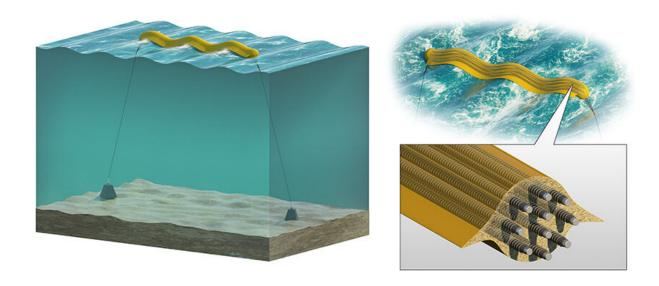
Distributed embedded energy converter technologies (or DEEC-Tecs) can be built into numerous shapes, like snakes and balloons, to capture energy from a wide range of ocean environments. Credit: Besiki Kazaishvili, NREL
