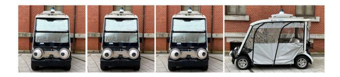
The cart was fitted with robotic eyes which could be moved in any direction, controlled by one of the research team. The windshield was covered to give the impression that there was no driver inside. Credit: Chang et al. 2022
