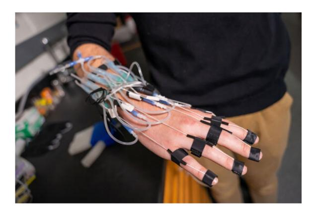
Rice University student Colter Decker, a senior majoring in mechanical engineering, demonstrates a glove that was used to demonstrate the analog features of soft pneumatic control circuitry for soft robotics. Credit: Brandon Martin/Rice University
