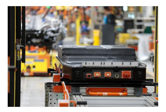
A battery waits to be installed on the frame of an electric-powered F-150 Lightning truck.
