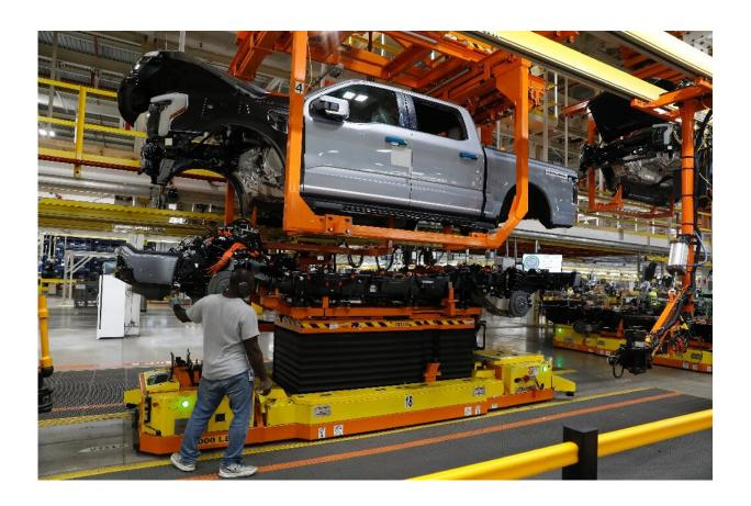
A cab is lowered on the frame of a battery-powered F-150 Lightning truck at Ford's Rouge Electric Vehicle Center in Dearborn, Michigan.
