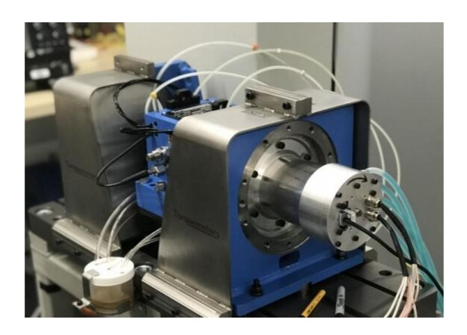
The new motor designed and built by the team at UNSW is an improvement on existing IPMSMs (Interior Permanent Magnet Synchronous Machine Motor), which are predominantly used in traction drive of electric vehicles. Credit: Dr Guoyo Chu
