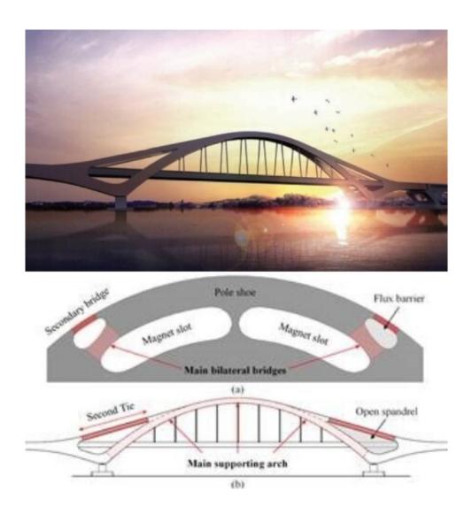
The design of the new IPMSM motor took its ispiration from the double-tied arch rail bridge in Gyopo, South Korea. Credit: Dr Guoyo Chu
