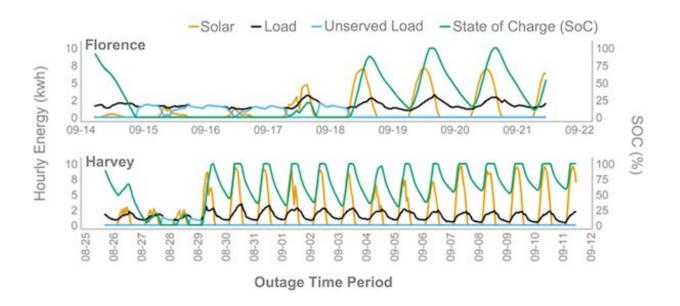
How a typical home would have done with solar and 30 kWh of storage after hurricanes Florence and Harvey. The light blue line shows the short periods of 'unserved load,' or shortfalls in meeting power demand, right after the storms. The state of charge shows batteries were able stretch solar power through the night. Credit: Berkeley Labs, <u>CC BY</u>
