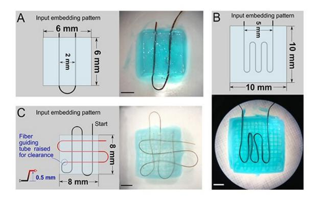
The input embedding pattern shows the fiber extruder being added to the hydrogel. Credit: Biohybrid and Organic Robotics Group, Carnegie Mellon University
