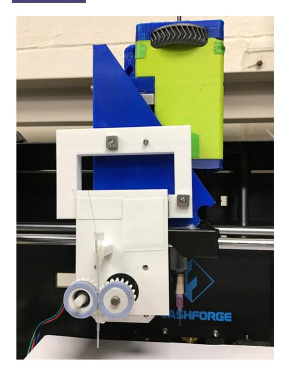
3D printing devices are crucial for enabling the fiber extruder to reinforce the hydrogel. Credit: Biohybrid and Organic Robotics Group
