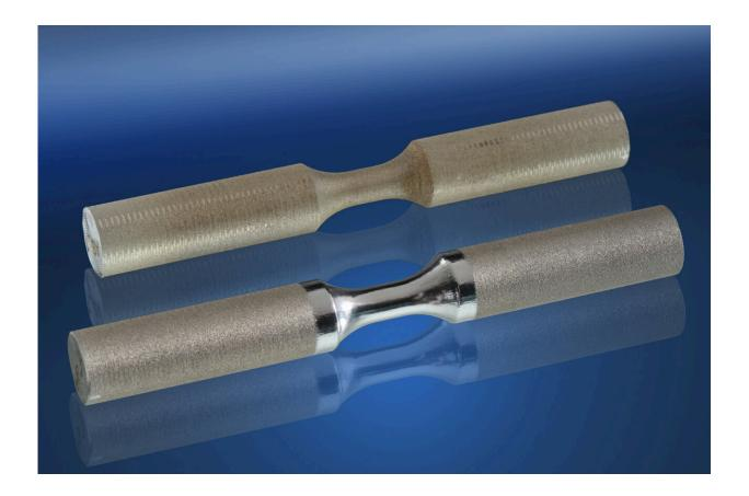
A barbell-shaped part made of stainless steel using a 3D printer and laser-polished in its middle section using the technique developed at Skoltech and MEPhI. These samples were used for metal fatigue testing. Credit: Daniil Panov/Skoltech.
