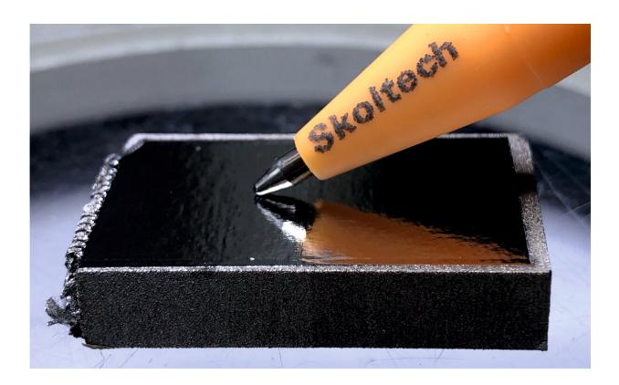
A stainless steel block manufactured with a 3D printer and laser-polished on top using the technique developed at Skoltech and MEPhI. Credit: Daniil Panov/Skoltech.
