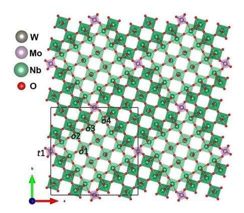
Full-sized image of the crystal structure of MWNO. The red, green, gray (in the faint-green octahedra) and purple spheres correspond to the O, Nb, W and Mo atoms in the unit cell, respectively. The structure consists of  $4 \times 4 \text{ ReO}_3$  blocks intersected with crystallographic shear planes. Credit: *Advanced Energy Materials* (2022). DOI: 10.1002/aenm.202200519
