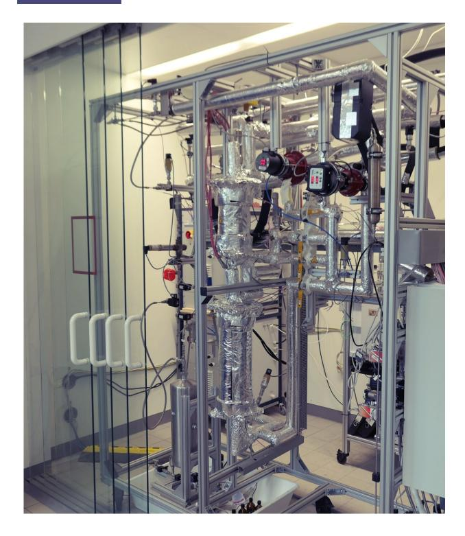
Methanol synthesis from metallurgical gases was successfully demonstrated in the miniplant. Credit: Fraunhofer ISE
